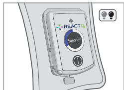
Charged Battery and Monitoring
